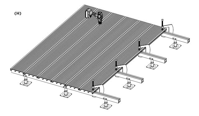
**12**. Fasten down the deck boards with black 30mm self-drill screws, through the AluClip, taking care not to scratch the top edges of the boards with the drill bit.
