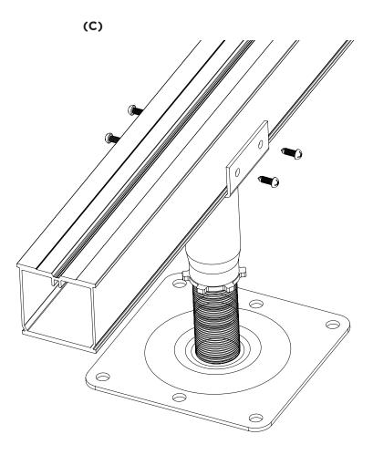
**3b.** OR; if using cleat supports, use the 4.8x19mm hex head self-drill screws to secure the joist at the required height. Note: in some scenarios, using packers to build up to the required height can be helpful. If the packers are not noncombustible, remove them after the screws have been installed. **Fig D.**
