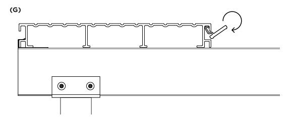
11. Optionally you can use G-clamps to lock the last row of deck boards tightly against previous rows, ensuring all gaps are consistent. **Fig H.**
