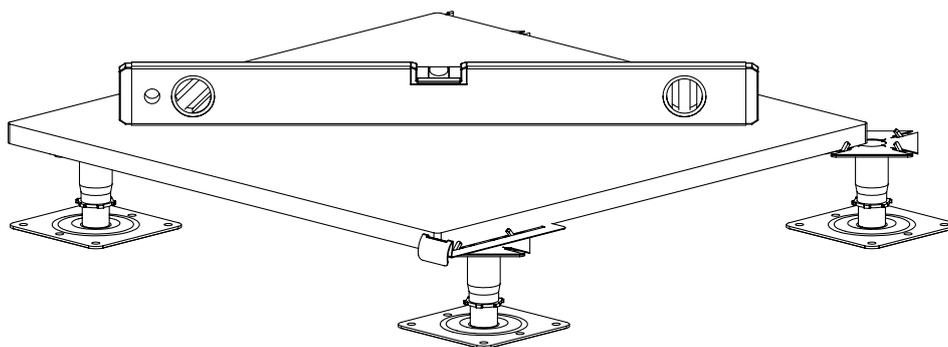
6. Position the next set of pedestals in place and lay slab on top. **Fig F.**
