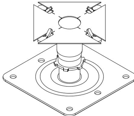
4. Place the first 4 pedestals in the desired area. When positioning pedestals along the perimeter of an area, ensure edge spring clips are used to create uniform spacing along these edges. **Fig D.**
