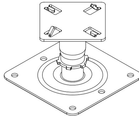
3. Place head rubber shockpads on top of pedestals. **Fig C.**
