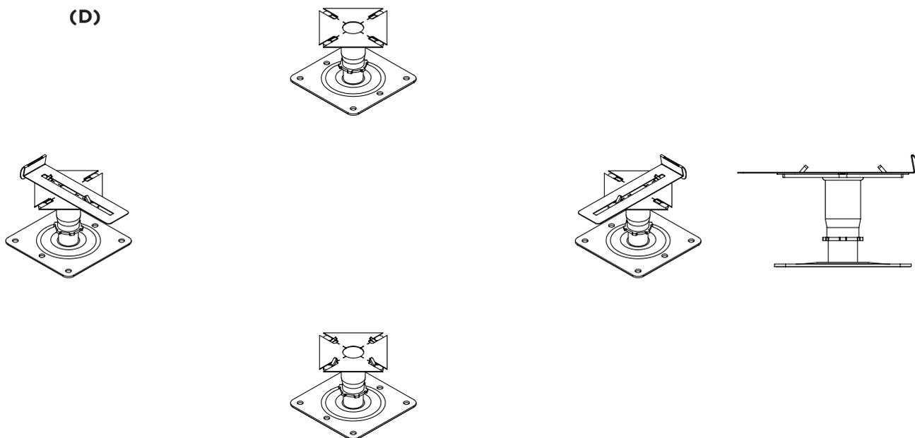
5. Lay slab on top of pedestals. Set the height of the slab and pedestals by placing a spirit level diagonally on the slab and twisting the pedestal upper shaft clockwise (down) or anti-clockwise (up). Tighten the locking nut to lock the pedestal height. **Fig E.**
