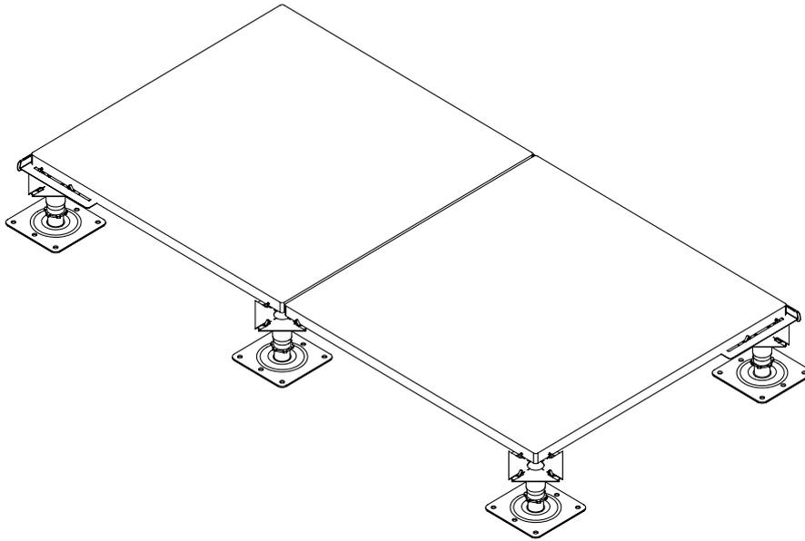
**7.** Level the slab with the previous by using a spirit level and raising/lowering the pedestals as described in point 5. If necessary, you can make minor adjustments to finished surface level by adding sections of head rubber shockpads beneath the tiles. **Fig G.**
